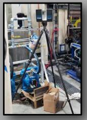
3D Laser Scanning Capability Using the FARO Focus Scanner
