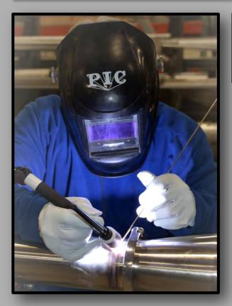
Piping Fabrication to ASME B31.3 Code
